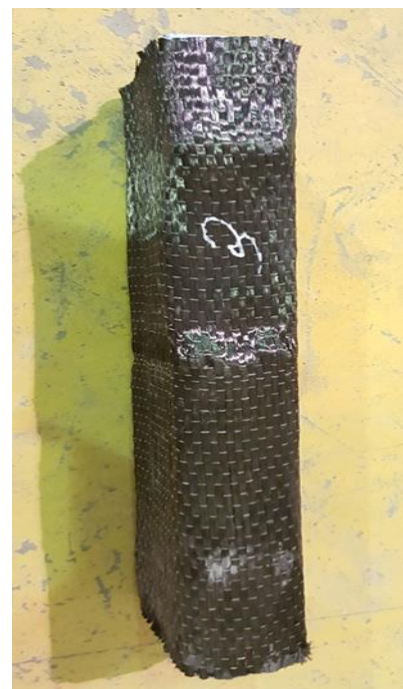
Fig. 2: CFRP wrapped box section
