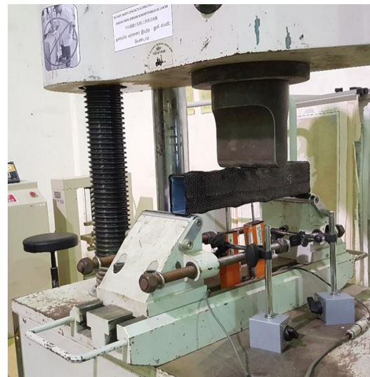
Fig. 6: Single point bending test of CFRP strengthened box section
